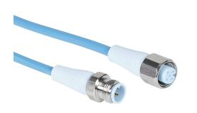
Murrelektronik connection cable, M12 axial male to M12 axial female, 4-pole, styrene-butadiene thermoplastic (TPE-S) jacket, ice blue, 9.8ft/3m cable length, IP65, IP68 and IP69K, suitable for food and beverage applications, FDA compliant.
