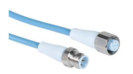
Murrelektronik connection cable, M12 axial male to M12 axial female, 4-pole, styrene-butadiene thermoplastic (TPE-S) jacket, ice blue, 3.2ft/1m cable length, IP65, IP68 and IP69K, suitable for food and beverage applications, FDA compliant.
