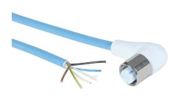
Murrelektronik connection cable, M12 right-angle female to pigtail, 5-pole, styrene-butadiene thermoplastic (TPE-S) jacket, ice blue, 65.6ft/20m cable length, IP65, IP68 and IP69K, suitable for food and beverage applications, FDA compliant.
