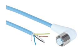
Murrelektronik connection cable, M12 right-angle female to pigtail, 5-pole, styrene-butadiene thermoplastic (TPE-S) jacket, ice blue, 49.2ft/15m cable length, IP65, IP68 and IP69K, suitable for food and beverage applications, FDA compliant.
