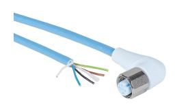
Murrelektronik connection cable, M12 right-angle female to pigtail, 5-pole, styrene-butadiene thermoplastic (TPE-S) jacket, ice blue, 32.8ft/10m cable length, IP65, IP68 and IP69K, suitable for food and beverage applications, FDA compliant.
