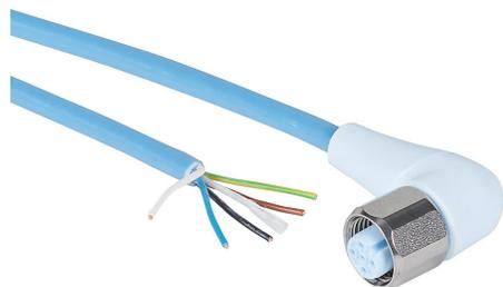
Murrelektronik connection cable, M12 right-angle female to pigtail, 5-pole, styrene-butadiene thermoplastic (TPE-S) jacket, ice blue, 32.8ft/10m cable length, IP65, IP68 and IP69K, suitable for food and beverage applications, FDA compliant.
