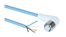
Murrelektronik connection cable, M12 right-angle female to pigtail, 5-pole, styrene-butadiene thermoplastic (TPE-S) jacket, ice blue, 22.9ft/7m cable length, IP65, IP68 and IP69K, suitable for food and beverage applications, FDA compliant.
