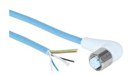
Murrelektronik connection cable, M12 right-angle female to pigtail, 5-pole, styrene-butadiene thermoplastic (TPE-S) jacket, ice blue, 16.4ft/5m cable length, IP65, IP68 and IP69K, suitable for food and beverage applications, FDA compliant.
