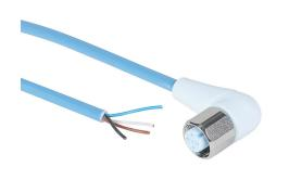
Murrelektronik connection cable, M12 right-angle female to pigtail, 4-pole, styrene-butadiene thermoplastic (TPE-S) jacket, ice blue, 82ft/25m cable length, IP65, IP68 and IP69K, suitable for food and beverage applications, FDA compliant.
