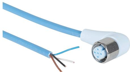
Murrelektronik connection cable, M12 right-angle female to pigtail, 4-pole, styrene-butadiene thermoplastic (TPE-S) jacket, ice blue, 65.6ft/20m cable length, IP65, IP68 and IP69K, suitable for food and beverage applications, FDA compliant.
