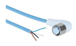
Murrelektronik connection cable, M12 right-angle female to pigtail, 4-pole, styrene-butadiene thermoplastic (TPE-S) jacket, ice blue, 65.6ft/20m cable length, IP65, IP68 and IP69K, suitable for food and beverage applications, FDA compliant.
