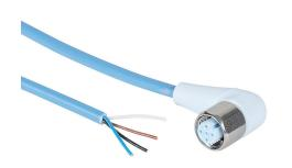
Murrelektronik connection cable, M12 right-angle female to pigtail, 4-pole, styrene-butadiene thermoplastic (TPE-S) jacket, ice blue, 32.8ft/10m cable length, IP65, IP68 and IP69K, suitable for food and beverage applications, FDA compliant.
