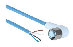
Murrelektronik connection cable, M12 right-angle female to pigtail, 4-pole, styrene-butadiene thermoplastic (TPE-S) jacket, ice blue, 22.9ft/7m cable length, IP65, IP68 and IP69K, suitable for food and beverage applications, FDA compliant.
