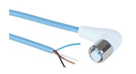
Murrelektronik connection cable, M12 right-angle female to pigtail, 4-pole, styrene-butadiene thermoplastic (TPE-S) jacket, ice blue, 16.4ft/5m cable length, IP65, IP68 and IP69K, suitable for food and beverage applications, FDA compliant.
