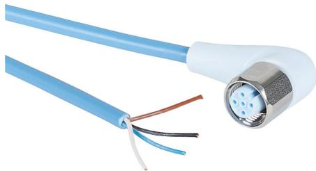
Murrelektronik connection cable, M12 right-angle female to pigtail, 4-pole, styrene-butadiene thermoplastic (TPE-S) jacket, ice blue, 9.8ft/3m cable length, IP65, IP68 and IP69K, suitable for food and beverage applications, FDA compliant.
