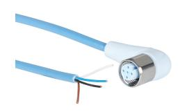
Murrelektronik connection cable, M12 right-angle female to pigtail, 4-pole, styrene-butadiene thermoplastic (TPE-S) jacket, ice blue, 6.5ft/2m cable length, IP65, IP68 and IP69K, suitable for food and beverage applications, FDA compliant.
