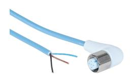
Murrelektronik connection cable, M12 right-angle female to pigtail, 3-pole, styrene-butadiene thermoplastic (TPE-S) jacket, ice blue, 16.4ft/5m cable length, IP65, IP68 and IP69K, suitable for food and beverage applications, FDA compliant.
