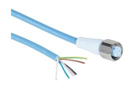
Murrelektronik connection cable, M12 axial female to pigtail, 5-pole, styrene-butadiene thermoplastic (TPE-S) jacket, ice blue, 65.6ft/20m cable length, IP65, IP68 and IP69K, suitable for food and beverage applications, FDA compliant.
