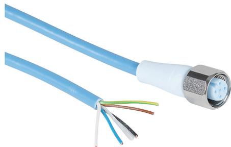
Murrelektronik connection cable, M12 axial female to pigtail, 5-pole, styrene-butadiene thermoplastic (TPE-S) jacket, ice blue, 65.6ft/20m cable length, IP65, IP68 and IP69K, suitable for food and beverage applications, FDA compliant.
