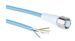
Murrelektronik connection cable, M12 axial female to pigtail, 5-pole, styrene-butadiene thermoplastic (TPE-S) jacket, ice blue, 49.2ft/15m cable length, IP65, IP68 and IP69K, suitable for food and beverage applications, FDA compliant.
