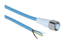
Murrelektronik connection cable, M12 axial female to pigtail, 5-pole, styrene-butadiene thermoplastic (TPE-S) jacket, ice blue, 32.8ft/10m cable length, IP65, IP68 and IP69K, suitable for food and beverage applications, FDA compliant.
