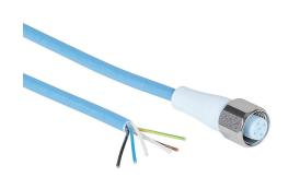
Murrelektronik connection cable, M12 axial female to pigtail, 5-pole, styrene-butadiene thermoplastic (TPE-S) jacket, ice blue, 16.4ft/5m cable length, IP65, IP68 and IP69K, suitable for food and beverage applications, FDA compliant.
