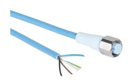
Murrelektronik connection cable, M12 axial female to pigtail, 5-pole, styrene-butadiene thermoplastic (TPE-S) jacket, ice blue, 9.8ft/3m cable length, IP65, IP68 and IP69K, suitable for food and beverage applications, FDA compliant.
