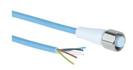
Murrelektronik connection cable, M12 axial female to pigtail, 5-pole, styrene-butadiene thermoplastic (TPE-S) jacket, ice blue, 6.5ft/2m cable length, IP65, IP68 and IP69K, suitable for food and beverage applications, FDA compliant.
