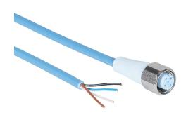
Murrelektronik connection cable, M12 axial female to pigtail, 4-pole, styrene-butadiene thermoplastic (TPE-S) jacket, ice blue, 32.8ft/10m cable length, IP65, IP68 and IP69K, suitable for food and beverage applications, FDA compliant.
