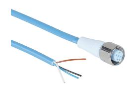
Murrelektronik connection cable, M12 axial female to pigtail, 4-pole, styrene-butadiene thermoplastic (TPE-S) jacket, ice blue, 16.4ft/5m cable length, IP65, IP68 and IP69K, suitable for food and beverage applications, FDA compliant.
