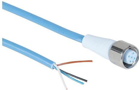
Murrelektronik connection cable, M12 axial female to pigtail, 4-pole, styrene-butadiene thermoplastic (TPE-S) jacket, ice blue, 16.4ft/5m cable length, IP65, IP68 and IP69K, suitable for food and beverage applications, FDA compliant.
