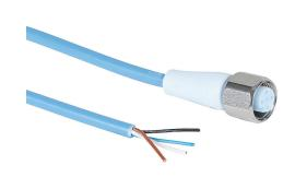
Murrelektronik connection cable, M12 axial female to pigtail, 4-pole, styrene-butadiene thermoplastic (TPE-S) jacket, ice blue, 9.8ft/3m cable length, IP65, IP68 and IP69K, suitable for food and beverage applications, FDA compliant.
