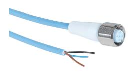
Murrelektronik connection cable, M12 axial female to pigtail, 3-pole, styrene-butadiene thermoplastic (TPE-S) jacket, ice blue, 16.4ft/5m cable length, IP65, IP68 and IP69K, suitable for food and beverage applications, FDA compliant.
