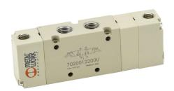
Metal Work pilot valve, 5-port (4-way), 3-position, center exhaust, double air pilot, 1/4in female NPT inlet(s), 1/4in female NPT outlet(s), 1/4in female NPT exhaust(s), 1/8in female NPT pilot(s), Cv=1.1.
