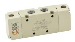
Metal Work pilot valve, 5-port (4-way), 2-position, double air pilot, 1/4in female NPT inlet(s), 1/4in female NPT outlet(s), 1/4in female NPT pilot(s), Cv=1.1.
