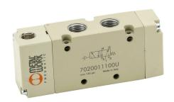
Metal Work pilot valve, 5-port (4-way), 2-position, single air pilot spring return, 1/4in female NPT inlet(s), 1/4in female NPT outlet(s), 1/4in female NPT exhaust(s), 1/8in female NPT pilot(s), Cv=1.1.
