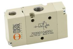
Metal Work pilot valve, 3-port (3-way), 2-position, N.O., single air pilot spring return, 1/4in female NPT inlet(s), 1/4in female NPT outlet(s), 1/4in female NPT exhaust(s), 1/8in female NPT pilot(s), Cv=1.1.
