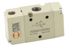
Metal Work pilot valve, 3-port (3-way), 2-position, N.C., single air pilot spring return, 1/4in female NPT inlet(s), 1/4in female NPT outlet(s), 1/4in female NPT exhaust(s), 1/8in female NPT pilot(s), Cv=1.1.
