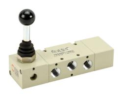
Metal Work pneumatic manual valve, 5-port (4-way), 3-position, center pressure, 90 deg hand lever, spring return, 1/4in female NPT inlet(s), 1/4in female NPT outlet(s), 1/4in female NPT exhaust(s), Cv=1.1.
