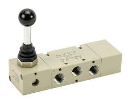
Metal Work pneumatic manual valve, 5-port (4-way), 3-position, center closed, 90 deg hand lever, spring return, 1/4in female NPT inlet(s), 1/4in female NPT outlet(s), 1/4in female NPT exhaust(s), Cv=1.1.
