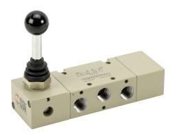
Metal Work pneumatic manual valve, 5-port (4-way), 3-position, center exhaust, 90 deg hand lever, spring return, 1/4in female NPT inlet(s), 1/4in female NPT outlet(s), 1/4in female NPT exhaust(s), Cv=1.1.
