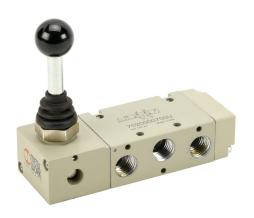
Metal Work manual valve, 5-port (4-way), 3-position, center pressure, 90 deg hand lever, detented, 1/4in female NPT inlet(s), 1/4in female NPT outlet(s), 1/4in female NPT exhaust(s), Cv=1.1.
