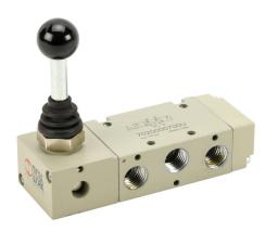
Metal Work pneumatic manual valve, 5-port (4-way), 3-position, center pressure, 90 deg hand lever, detented, 1/4in female NPT inlet(s), 1/4in female NPT outlet(s), 1/4in female NPT exhaust(s), Cv=1.1.
