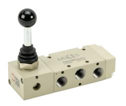
Metal Work pneumatic manual valve, 5-port (4-way), 3-position, center exhaust, 90 deg hand lever, detented, 1/4in female NPT inlet(s), 1/4in female NPT outlet(s), 1/4in female NPT exhaust(s), Cv=1.1.
