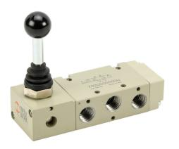
Metal Work pneumatic manual valve, 5-port (4-way), 3-position, center closed, 90 deg hand lever, detented, 1/4in female NPT inlet(s), 1/4in female NPT outlet(s), 1/4in female NPT exhaust(s), Cv=1.1.
