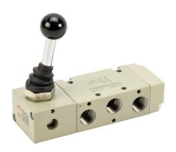
Metal Work pneumatic manual valve, 5-port (4-way), 2-position, 90 deg hand lever, detented, 1/4in female NPT inlet(s), 1/4in female NPT outlet(s), 1/4in female NPT exhaust(s), Cv=1.1.
