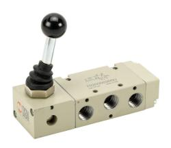
Metal Work pneumatic manual valve, 5-port (4-way), 2-position, 90 deg hand lever, spring return, 1/4in female NPT inlet(s), 1/4in female NPT outlet(s), 1/4in female NPT exhaust(s), Cv=1.1.
