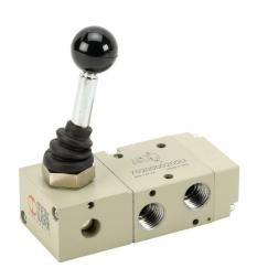
Metal Work pneumatic manual valve, 3-port (3-way), 2-position, 90 deg hand lever, detented, 1/4in female NPT inlet(s), 1/4in female NPT outlet(s), 1/4in female NPT exhaust(s), Cv=1.1.
