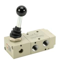
Metal Work pneumatic manual valve, 3-port (3-way), 2-position, N.C., 90 deg hand lever, spring return, 1/4in female NPT inlet(s), 1/4in female NPT outlet(s), 1/4in female NPT exhaust(s), Cv=1.1.
