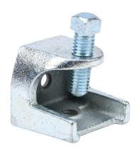
Minerallac screw-on beam clamp, 750 lbs. Package of 6. For use with flanges up to 3/4in and 3/8-16 threaded rod.
