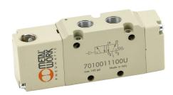
Metal Work pilot valve, 5-port (4-way), 2-position, single air pilot spring return, 1/8in female NPT inlet(s), 1/8in female NPT outlet(s), 1/8in female NPT exhaust(s), 1/8in female NPT pilot(s), Cv=0.55.
