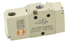
Metal Work pilot valve, 3-port (3-way), 2-position, N.O., single air pilot spring return, 1/8in female NPT inlet(s), 1/8in female NPT outlet(s), 1/8in female NPT exhaust(s), 1/8in female NPT pilot(s), Cv=0.55.
