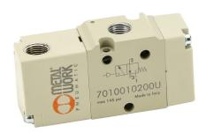
Metal Work pilot valve, 3-port (3-way), 2-position, N.C., single air pilot spring return, 1/8in female NPT inlet(s), 1/8in female NPT outlet(s), 1/8in female NPT exhaust(s), 1/8in female NPT pilot(s), Cv=0.55.
