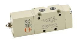
Metal Work pneumatic mechanically operated directional control valve, 5-port (4-way), 2-position, pneumatic switch, spring return, 1/8in female NPT inlet(s), 1/8in female NPT outlet(s), 1/8in female NPT exhaust(s), Cv=0.55.
