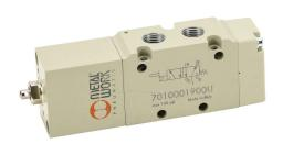
Metal Work mechanically operated directional control valve, 5-port (4-way), 2-position, pneumatic switch, spring return, 1/8in female NPT inlet(s), 1/8in female NPT outlet(s), 1/8in female NPT exhaust(s), Cv=0.55.
