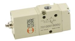
Metal Work pneumatic mechanically operated directional control valve, 3-port (3-way), 2-position, N.C., pneumatic switch, spring return, 1/8in female NPT inlet(s), 1/8in female NPT outlet(s), 1/8in female NPT exhaust(s), Cv=0.55.
