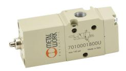
Metal Work mechanically operated directional control valve, 3-port (3-way), 2-position, N.C., pneumatic switch, spring return, 1/8in female NPT inlet(s), 1/8in female NPT outlet(s), 1/8in female NPT exhaust(s), Cv=0.55.
