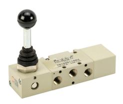
Metal Work pneumatic manual valve, 5-port (4-way), 3-position, center pressure, 90 deg hand lever, spring return, 1/8in female NPT inlet(s), 1/8in female NPT outlet(s), 1/8in female NPT exhaust(s), Cv=0.55.
