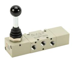
Metal Work pneumatic manual valve, 5-port (4-way), 3-position, center closed, 90 deg hand lever, spring return, 1/8in female NPT inlet(s), 1/8in female NPT outlet(s), 1/8in female NPT exhaust(s), Cv=0.55.
