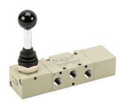
Metal Work pneumatic manual valve, 5-port (4-way), 3-position, center exhaust, 90 deg hand lever, spring return, 1/8in female NPT inlet(s), 1/8in female NPT outlet(s), 1/8in female NPT exhaust(s), Cv=0.55.
