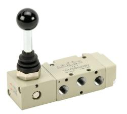
Metal Work pneumatic manual valve, 5-port (4-way), 3-position, center exhaust, 90 deg hand lever, detented, 1/8in female NPT inlet(s), 1/8in female NPT outlet(s), 1/8in female NPT exhaust(s), Cv=0.55.
